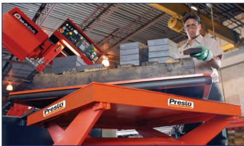
Standard Turntable shown mounted on Hydraulic Lift
