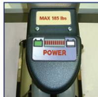
Battery indicator displays power level
